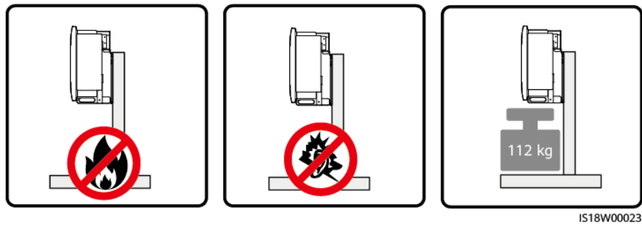
Figure 4-2 Mounting structure requirements
